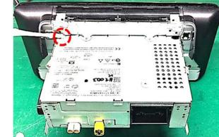
Attach the daughter PCB to the spacer. Connect the previously mounted 60-pin and the original ribbon cable to the ribbon cable bases "IN" / "OUT".
