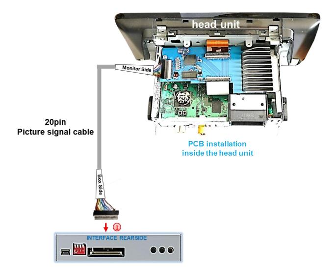
Connect the female 20pin connector of the daughter PCB's pre-connected 20pin picture signal cable to the video interface's male 20pin connector.
