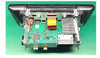
Unscrew the 5 screws on the top of the head unit and remove the housing cover.
