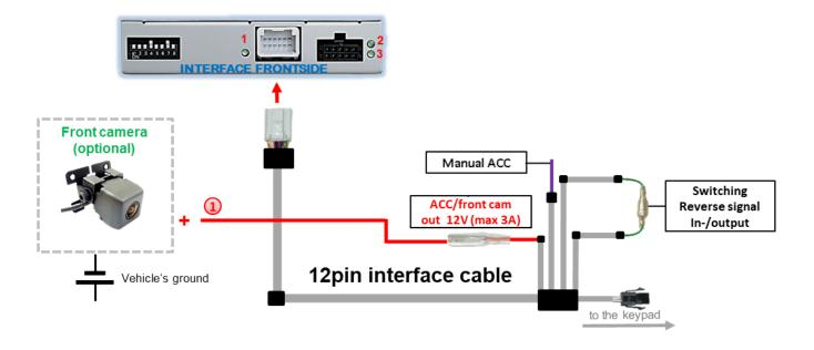
The red power supply output ACC/front cam out 12V (max 3A) can be used to power a front camera. If Dip 1 is set to ON (black 8 dips), the power supply output gives +12V (max 3A) when reverse gear is engaged plus 10 seconds delay after reverse gear is disengaged.
