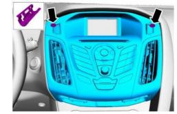
2. Carefully pop off the radio bezel making note that it is held by 2 clips as shown on the illustration above.
