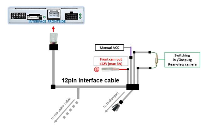
The red power supply output Front cam out +12V (max 3A) can be used to power a front cam with dip switch 1 (of the black 8 dips) to ON.
