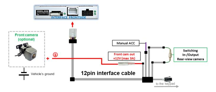
The red power supply output Front cam out +12V (max 3A) can be used to power a front camera. If Dip 1 is set to ON (black 8 dips), the power supply output gives +12V (max 3A) when reverse gear is engaged
