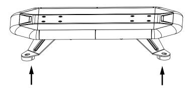
2. Put the lightbar on the car roof and tighten the four bolts of the two mounting feet.
