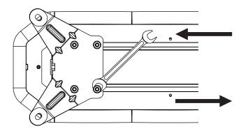
1. Put the two mouting feet onto the aluminium base. Adjust the two feet's distance to make the lightbar fit on the car roof. Then tighten the four bolts of each mounting foot.
