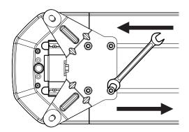
1. Put the two mouting feet onto the aluminium base. Adjust the two feet's distance to make the lightbar fit on the car roof. Then tighten the four bolts of each mounting foot.
