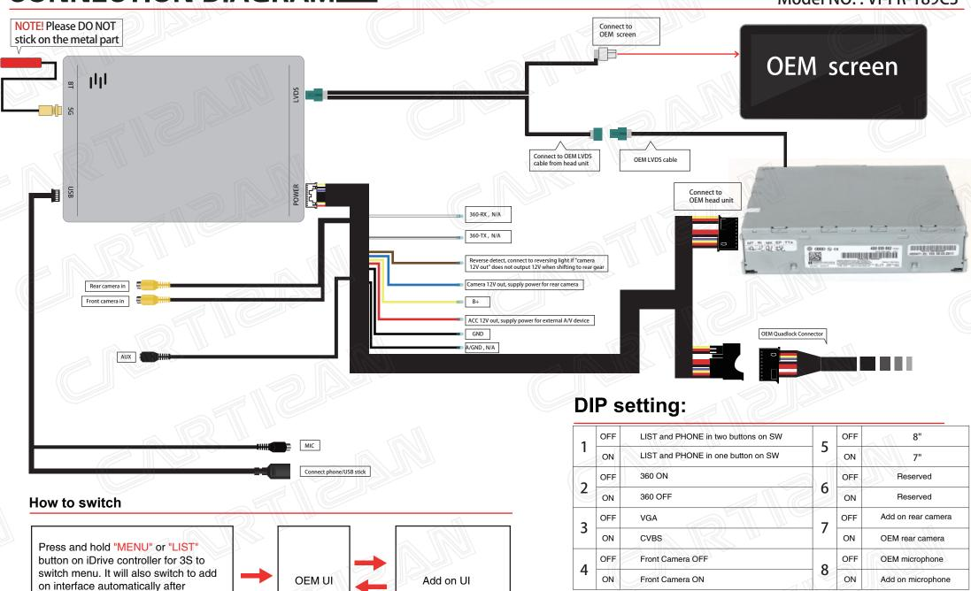
NOTE! Please try another car model DIP settings if your current car model DIP doesn't work. Disconnect and reconnect interface's power for effective after changing any DIP setting.
