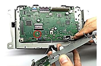
Carefully seperate the metal cover and disconnect the small Coaxial wire connected in between.
