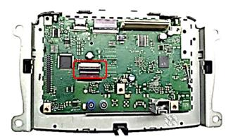
Disconnect the ribbon cable from the mainboard's ribbon cable base, as shown above.
