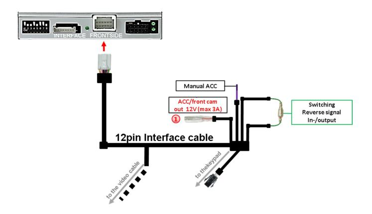
The red power supply output ACC/front cam out 12V (max 3A) can be used to power an external source and has a different assignment, depending on the position of dip switch 1 (of 8 dips):
