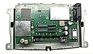
Carefully separate the original PCB from the system. Make sure not to damage the connector.
