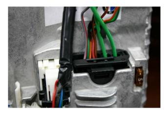
Disconnect the 12-pin plug insert from the black plug. This is best done using a fine slotted screwdriver to lift the catch.
