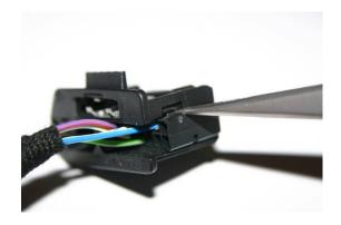
Push the 12-pin plug insert into the interface casing, in the direction of the arrows.
