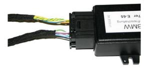
Plug the 12-pin insert on the interface into the original plug.
