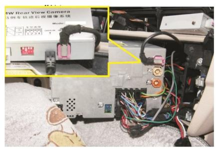
$\hbox{5.pry out the pink cable from original car and connected to LVDS-out put (see picture)}\\$
