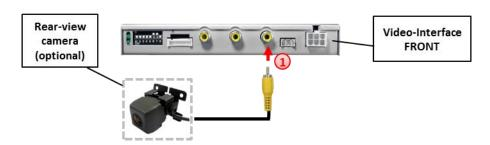
1 Connect the video-RCA of the after-market rear-view camera to the female RCA port of the video-interface which is labeled as CAM.
