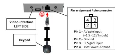
1 Connect the female 4pin Microfit connector of the keypad to the male 4pin Microfit connector of the video-interface.
