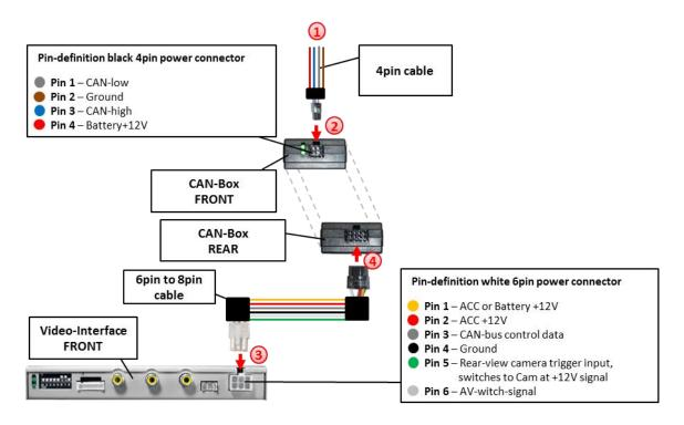
Connect CAN-bus and power at the rear of the factory monitor, otherwise no interface function! The connector can be different to the pictured connector.
